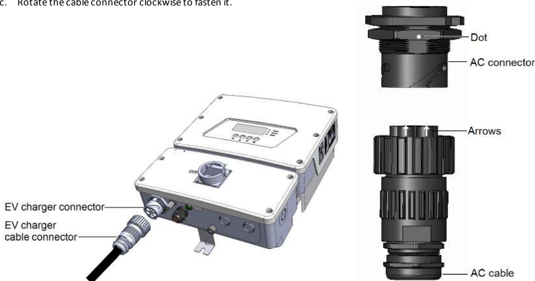
Figure 1: EV cable connection
